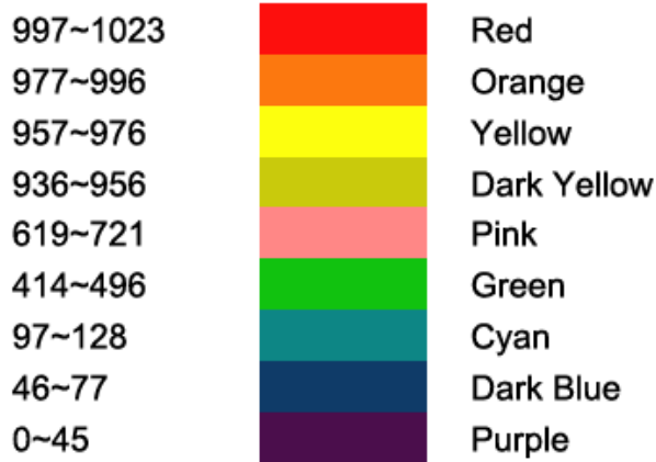
Figure 5.1-8 RED Mode- Mapping of Color and Luminance
